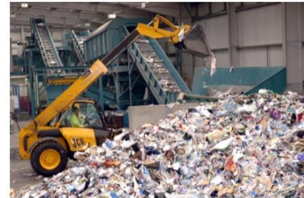
Recyclate sorting at a Materials Recovery Facility. Image copyright SEPA.
